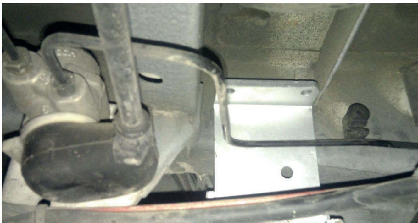
Insert the adapters, then drill the 10 mm holes (on both sides); finally insert and fix the connection bar.
