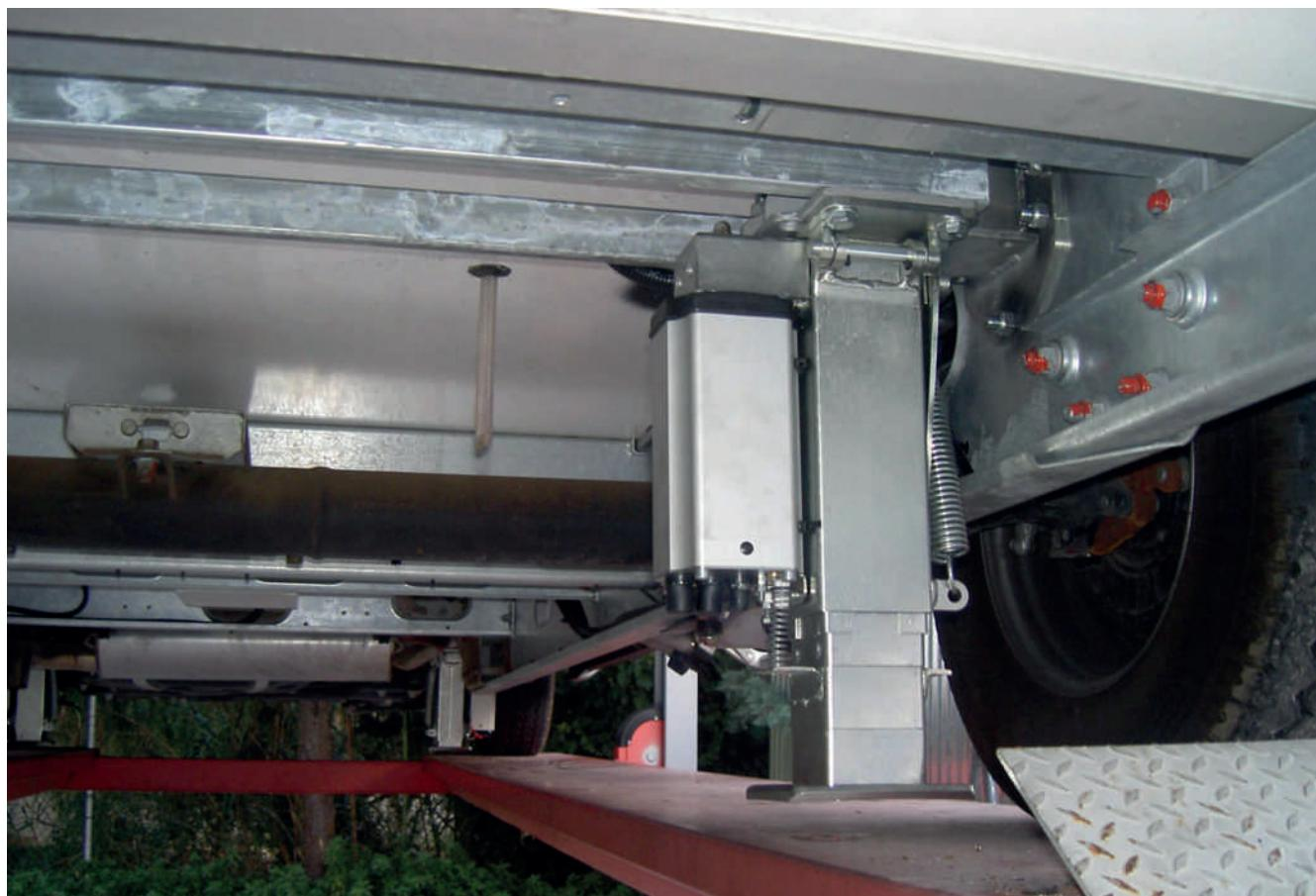
Beware: both jacks must be facing with the motor towards the rear, rotation towards the inside of the vehicle.
